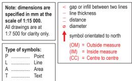
Most of the symbols in this specification shall be orientated to north. That a symbol is to be orientated to north is indicated with an arrow pointing upward beside the symbol. When a symbol shall be orientated to north, it means that it shall be orientated to magnetic north and hence relative to the edges of the paper and the magnetic north lines.
